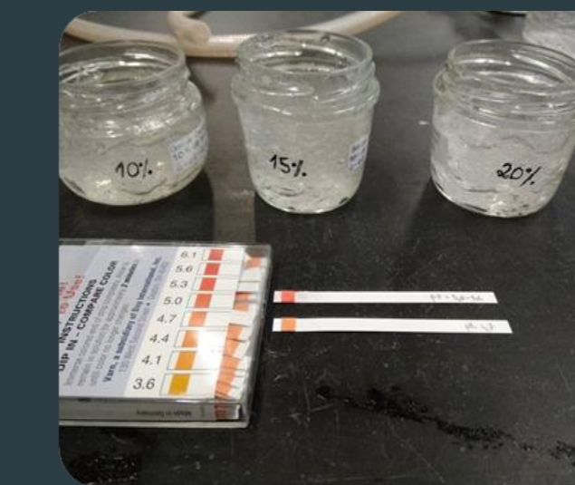
Fig 4 - Determination of the pH
