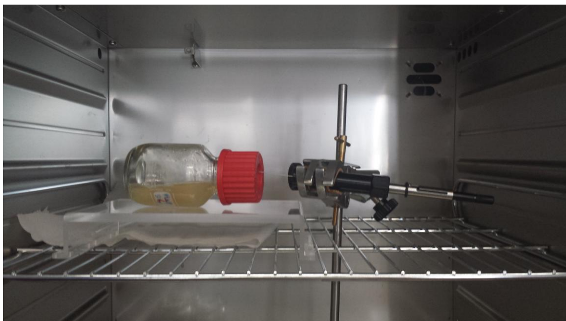
Figure S1 – In vitro fungal culture flasks (50 mL) sealed with a cap containing a silicone septum. This system was used to evaluate the production of volatile organic
