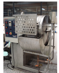
Fig 2 . Pilot drum used in the coating process
