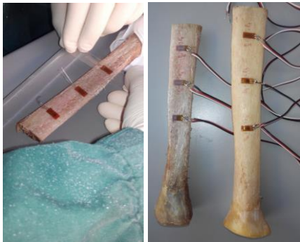
Fig. 3 Human samples instrumentation
