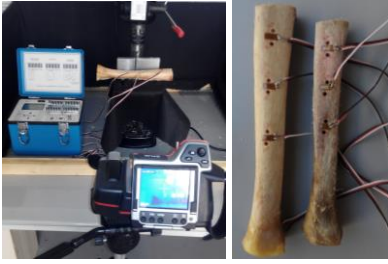
Fig. 4 Drilling tests on cadaveric tibiae
