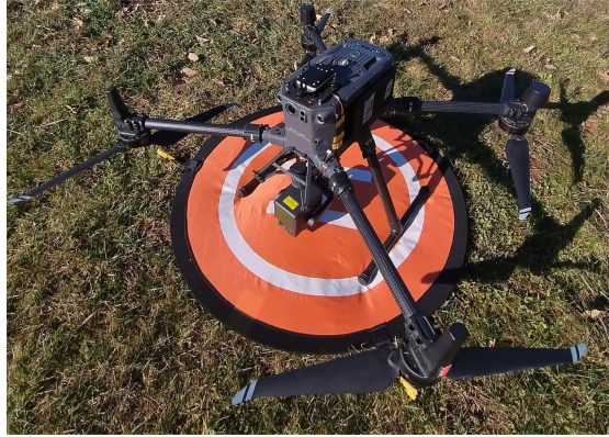
Fig. 2. The UAV-based LiDAR set employed to collect LiDAR data from the study site.
