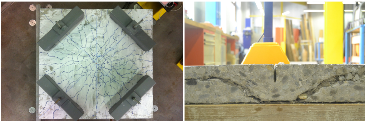
Fig. 9 Cracking pattern and internal shear crack of slab BC01 after failure.
