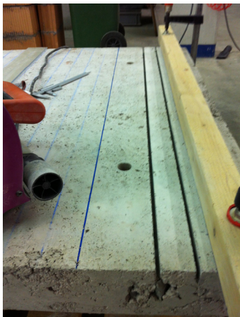
Fig. 6 BCN1 slots cutting.
