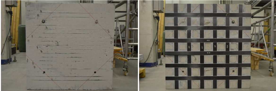
Fig. 11 Final aspect of BCN1 specimen after failure. Fig. 12 Final aspect of BCG1 specimen after failure.
