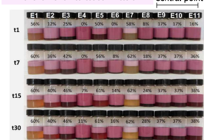
Fig. 2 Results of the 11 experimental runs (emulsions) obtained by the Central Composite Rotatable Design 22 for Creaming Index (CI) over time: t1; t7; t15, and t30.
