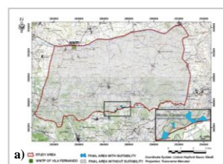
Image 1. Suitability map of soils for the infiltration of reclaimed water (a); Soil column in operation (b).
