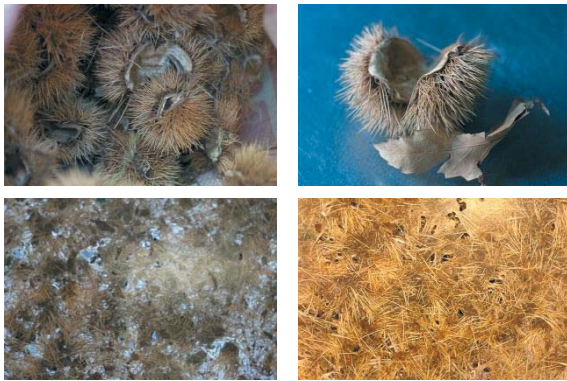
Fig. 1 - Chestnut hedgehogs (top-left); Chestnut hedgehog spikes (top-right); thermosetting resin plate and chestnut hedgehog spikes - plate photographed backlit (bottom-left); plate photographed with front light (bottom-right).
