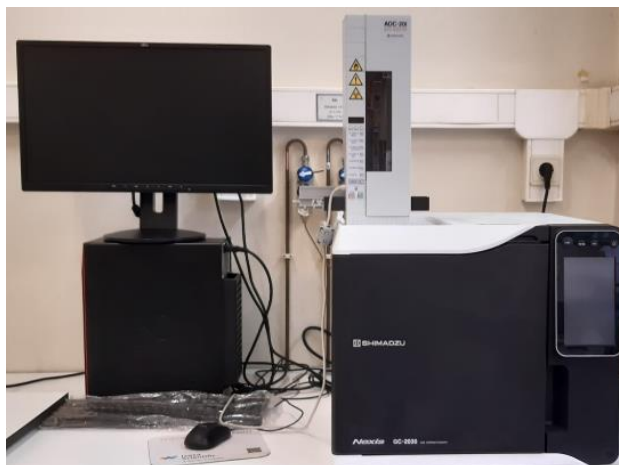
Figure 9. GC-FID equipment used for FAME content analysis in biodiesel samples.
