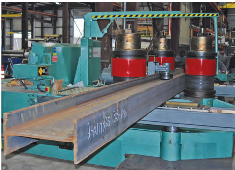
(a) Roller-bending of an I beam.
