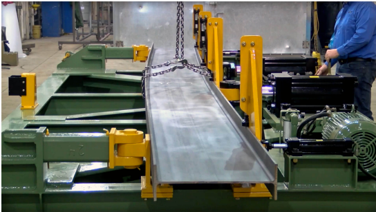
(a) Cold incremental cambering of an I-beam
