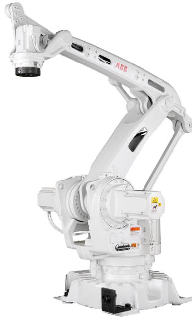
Figure 3.1: The ABB IRB 460 high-speed palletizing robot, known for its compact design and efficiency in end-of-line applications [21].
