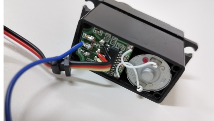
Figure 3.10: Adapted servo motor for absolute position sensing using the potentiometer.
