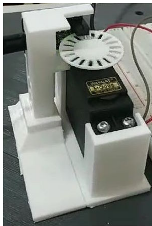
Figure 3.9: Custom-designed 3D-printed support structure for mounting the infrared sensor and servo motor.
