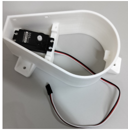
(a) Attaching the servo motor to the base support, enabling base rotation.
