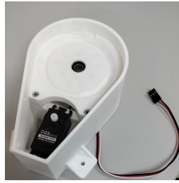
(b) Installing the main gear interacting with the base motor to drive rotation.
