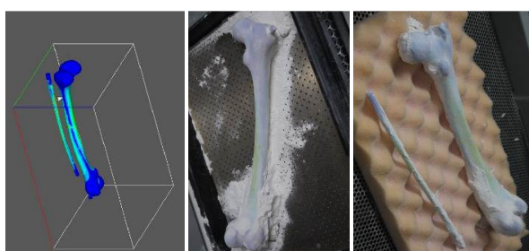
Fig. 14 - Main steps to fabricate the colour models
