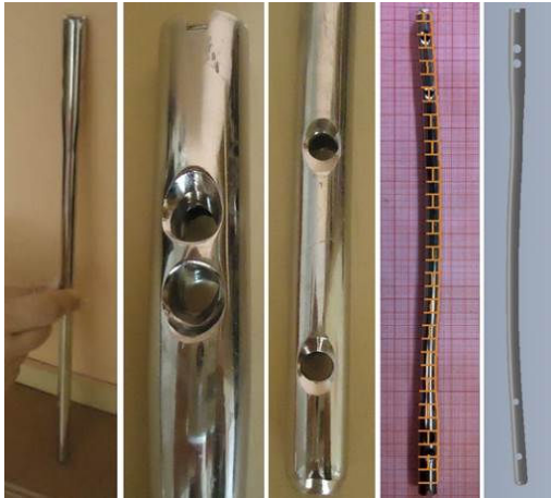
Fig. 4 - Intra-medullary nail and CAD model
