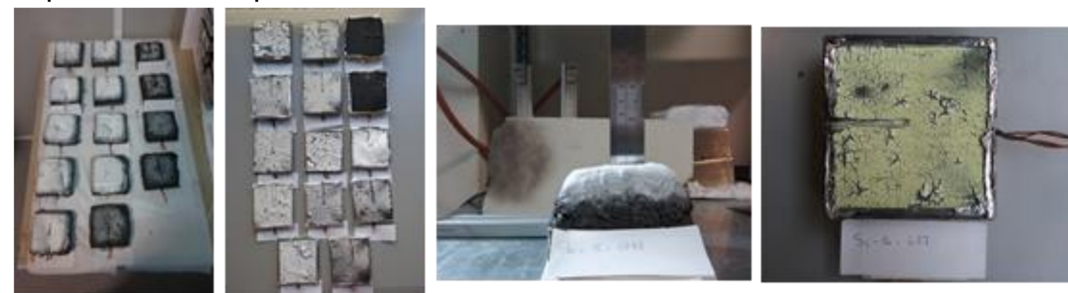
Coated steel plates before and after accelerated aging, with fixed thermocouples. Tested samples at 35 and 75 KW.m 2 .
