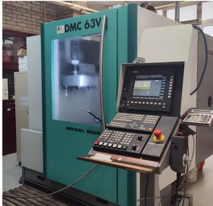
Figura 14 – Fresadora CNC – Deckel Maho DMC 63V.
