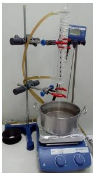
Figure III - Magnetic stirring plate IKA® C-MAG HS 7 with temperature control IKA® ETS-D5.
