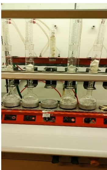
Figure 15: Total fat extraction process using Soxhlet equipment.
