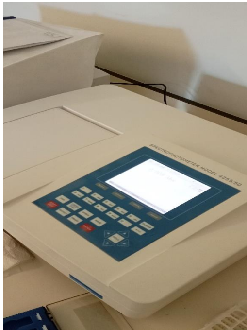
Figure 22: Zuzi spectrophotometer model 4255/50 used during \beta -glucan analysis.
