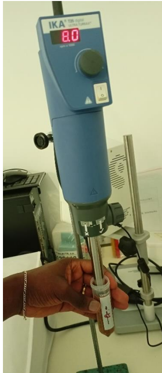
Figure 18: Sporocarp sample being homogenized using an IKA digital ultraturax before IND experiments.
