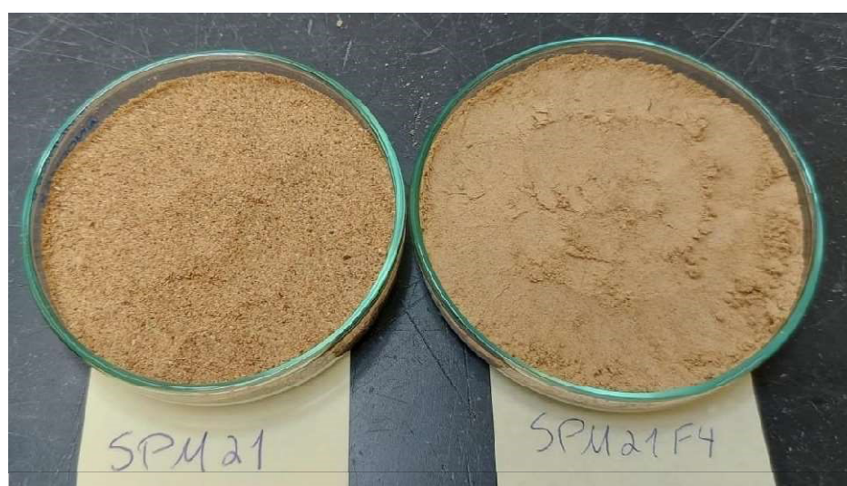
Figure 6. Representative image of the 2 samples analyzed. On the left, the untreated sample (SPM21) and on the right, the sample treated to reduce tannins (SPM21F4).
