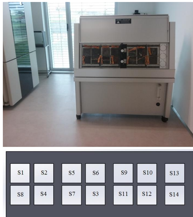
Figure 21: Position of specimens inside QUV Accelerated Weathering Tester.
