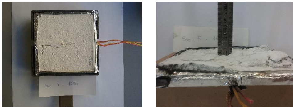
Figure 31: Final intumescent char thickness of specimen S10.
