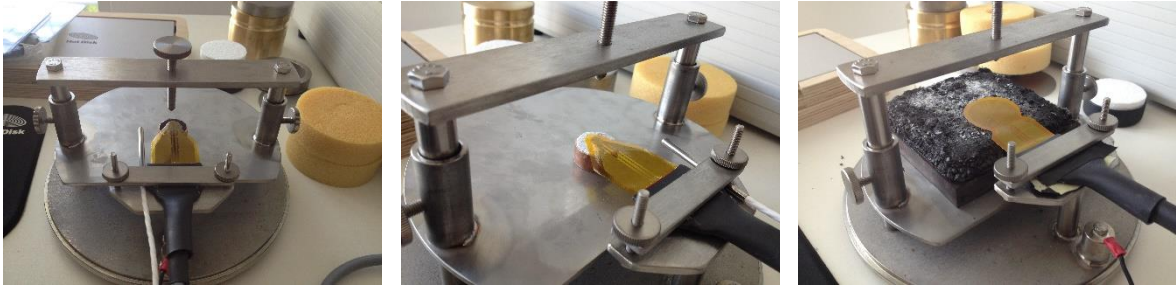
Figure 33: Measured thermal conductivity of intumescent char before and after aging using HotDisk.
