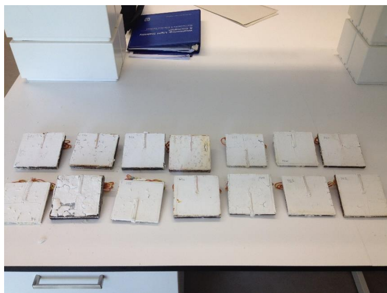
Figure 23: Intumescent coating surface after hydrothermal aging test of all specimens.
