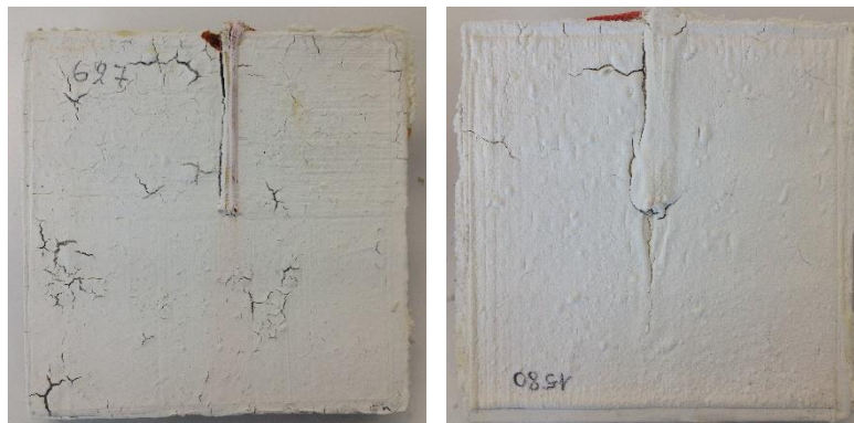
Figure 22: Intumescent coating surface after hydrothermal aging test of two different dry film thicknesses.
