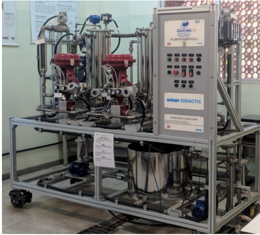
Figure 1: Illustration of the SMAR PD3 didactic plant
