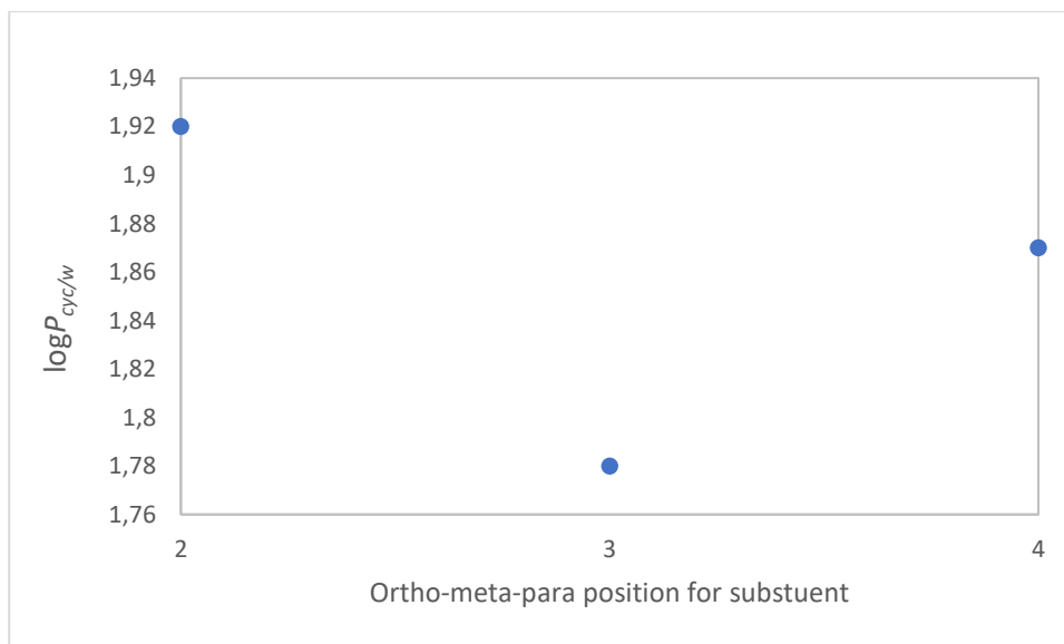
Figure 2.11 Evolution of \log P_{cyc/w} of methylbenzaldehyde according to the positions of the substituent.
