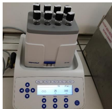
Figure 3.2 A) Glass graduated tubes; B) Thermostatic and shaking equipment (ThermoMixer C, Eppendorf)
