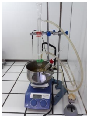
Figure 6. The experimental assembly used for esterification reactions.
