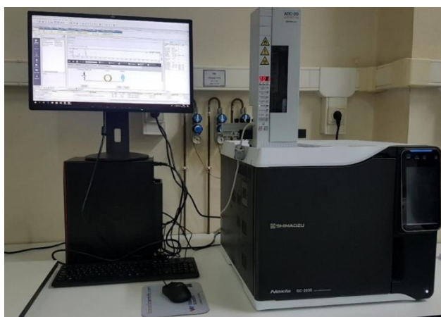
Figure 8. GC-FID equipment used to measure the content of FAMES in biodiesel samples.
