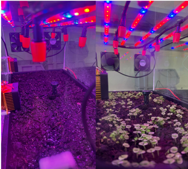
Figure 5.4: Cultivation Test: Left Side Shows the First Day, and Right Side Shows the Last Day.
