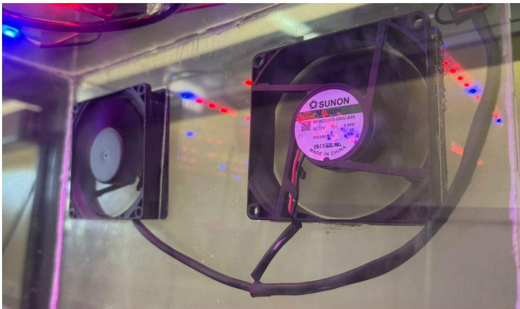
Figure 4.20: Ventilators in the Prototype.
