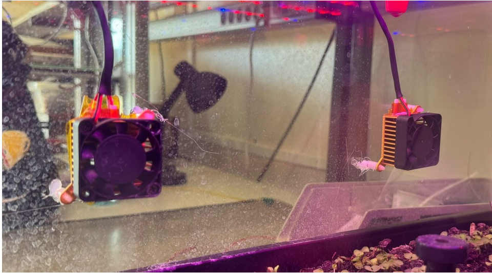
Figure 4.18: Heaters in the Prototype.
