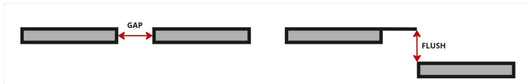
Figure 3.2: Schematic representation of the gap and flush parameters.
