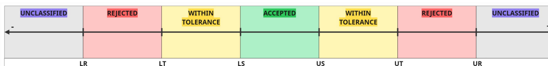
Figure 3.3: Measurement classification zones based on specified limits.
