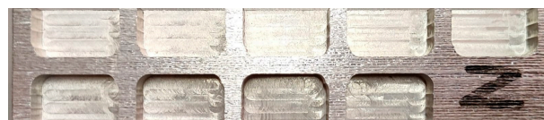
Figure 4. Zig-Zag milled pockets.
