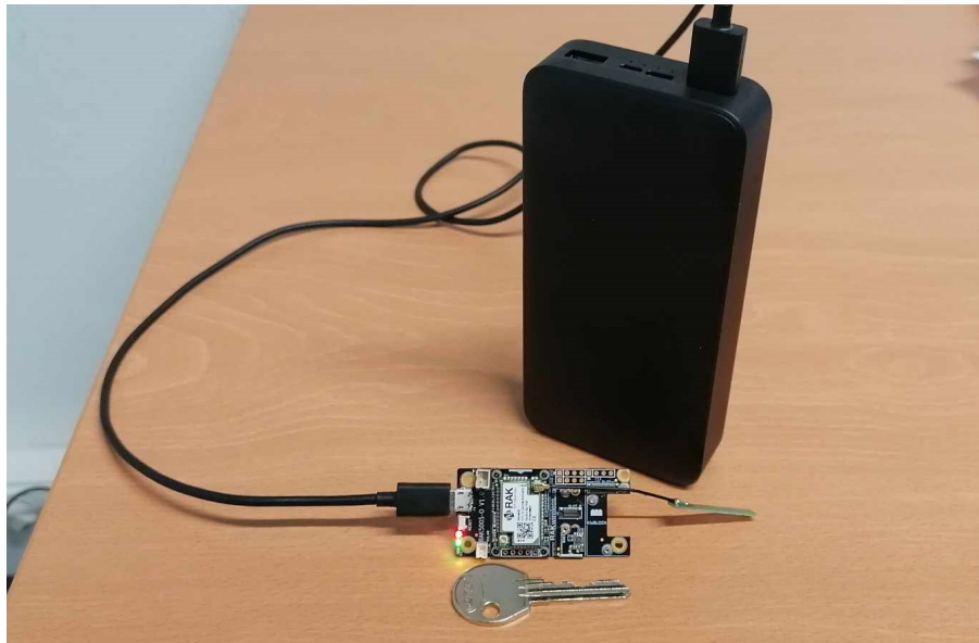
Figure 4.2: RAK4630 connected to Powerbank Xiaomi Redmi 2 20000mAh 18W [Author's Source]
