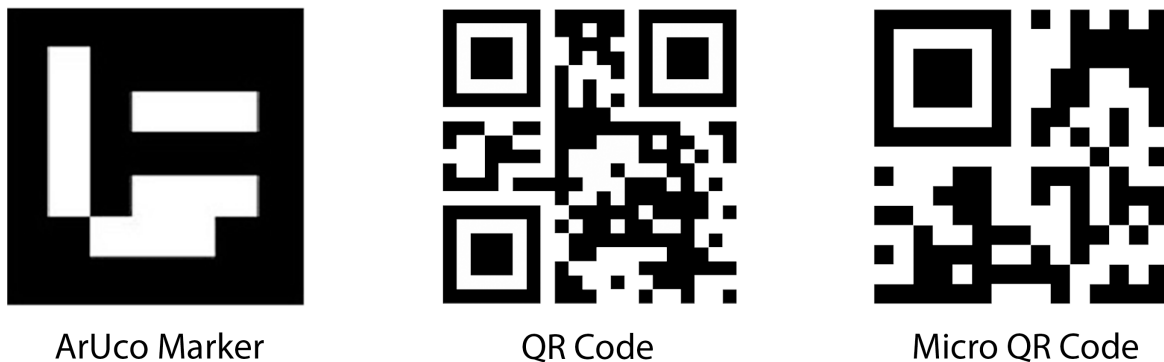
Figure 2.9: Example of ArUco Marker, QR Code and Micro QR Code [Author's Source]
