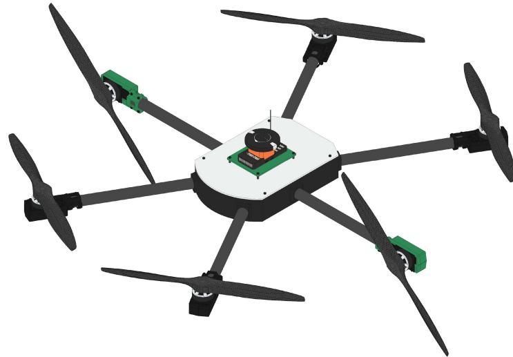
Figure 2. Proposed HTR with two servomotors tilted 90°.
