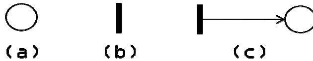
Figure 2-5- Objects in Petri Nets: (a) place, (b) transition, (c) arc connecting a transition to a place
