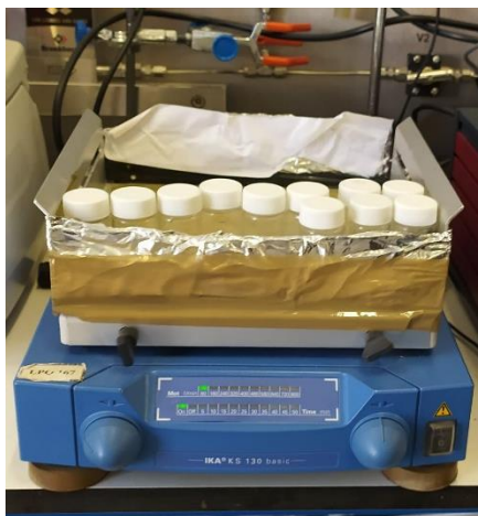
Figure 3 - Batch adsorption in an orbital shaker at room temperature.
