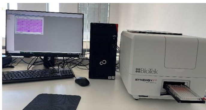
Figure 11. Microplate reader equipment to evaluate the anti-inflammatory activity.
