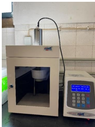
Figure 8. Ultrasound equipment used for UAE extraction.
