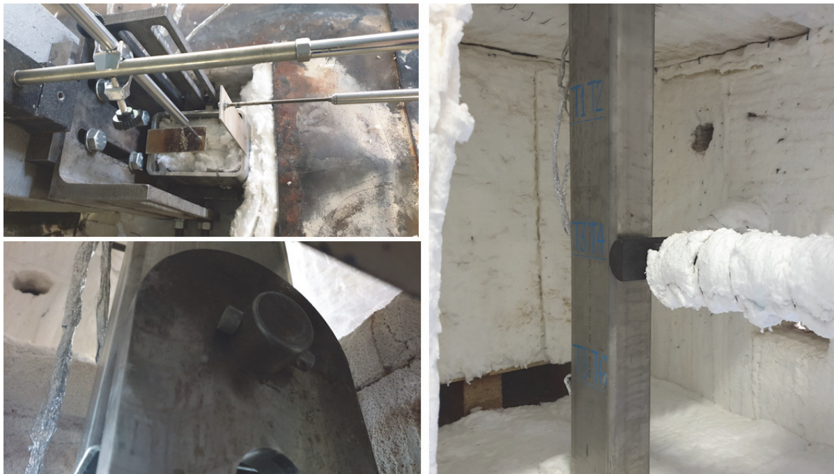
Fig. 2 – Beam inside the furnace and supporting conditions.
