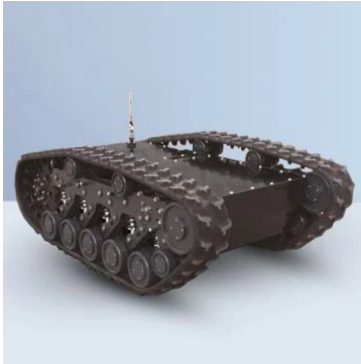
Figure 2.4: Tracked mobile robot (crawler-type chassis)
