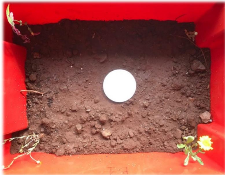
Figure 10. Container used for humidity level assays (50 x 40 x 40 cm).
