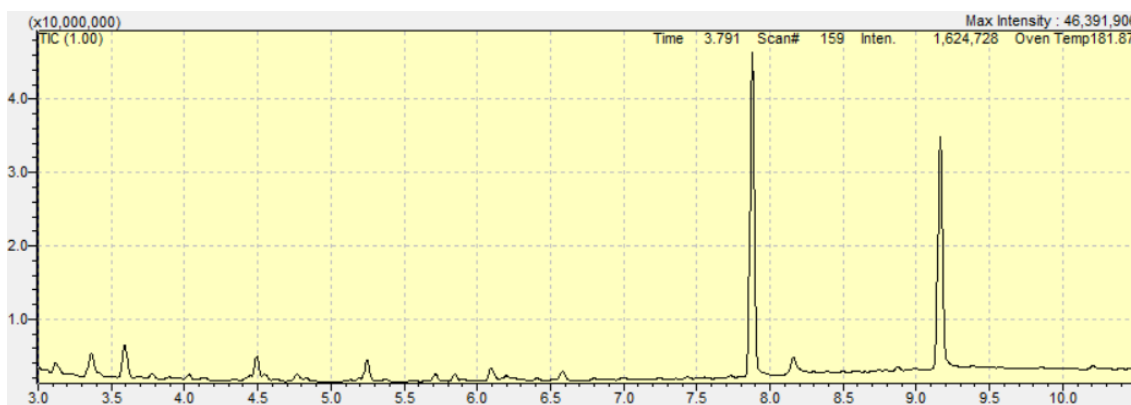
Figure 13. Blank MSTFA with 5% TMCS SCAN Chromatogram.
