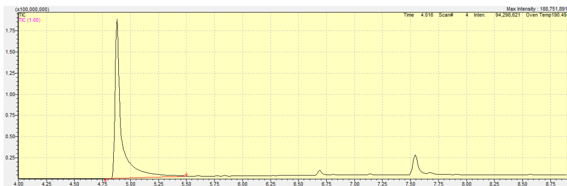
Figure 4. GC-MS chromatogram of 2,4-DNP standard (100 ppm) without derivatization, analyzed using the conditions of method #1.
