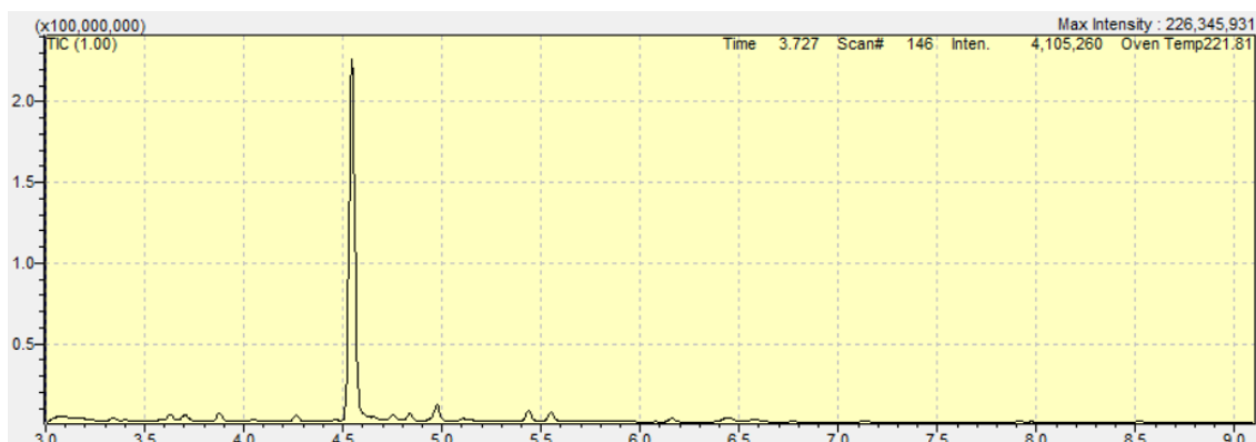
Figure 8. GC-MS chromatogram of 2,4-DNP standard (7.5 ppm) after derivatization with BSTFA w/ 1% TMCS using 60 minutes and 90°C derivatization.
