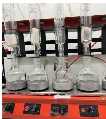
Figure 9. Total lipid extraction using Soxhlet apparatus.
