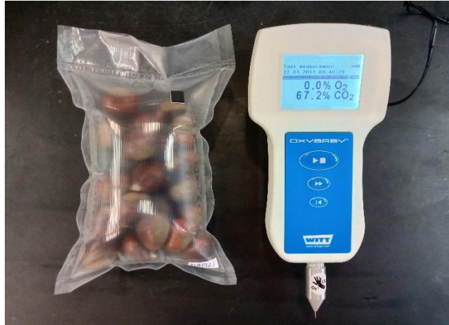
Figure 4: O 2 and CO 2 gas analyzer for Modified Atmosphere Packaging.
